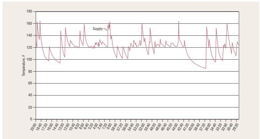
**FIGURE 2.** In this building, the plumber insisted that the newly installed indirect water heater did not need a return line, claiming that the indirect water heater in his building was absent a return line with no resulting temperature control problems. In reality, the temperature at the hot outlet is sometimes close to the setpoint of 120 F, but it is dangerously overheated at other times.
