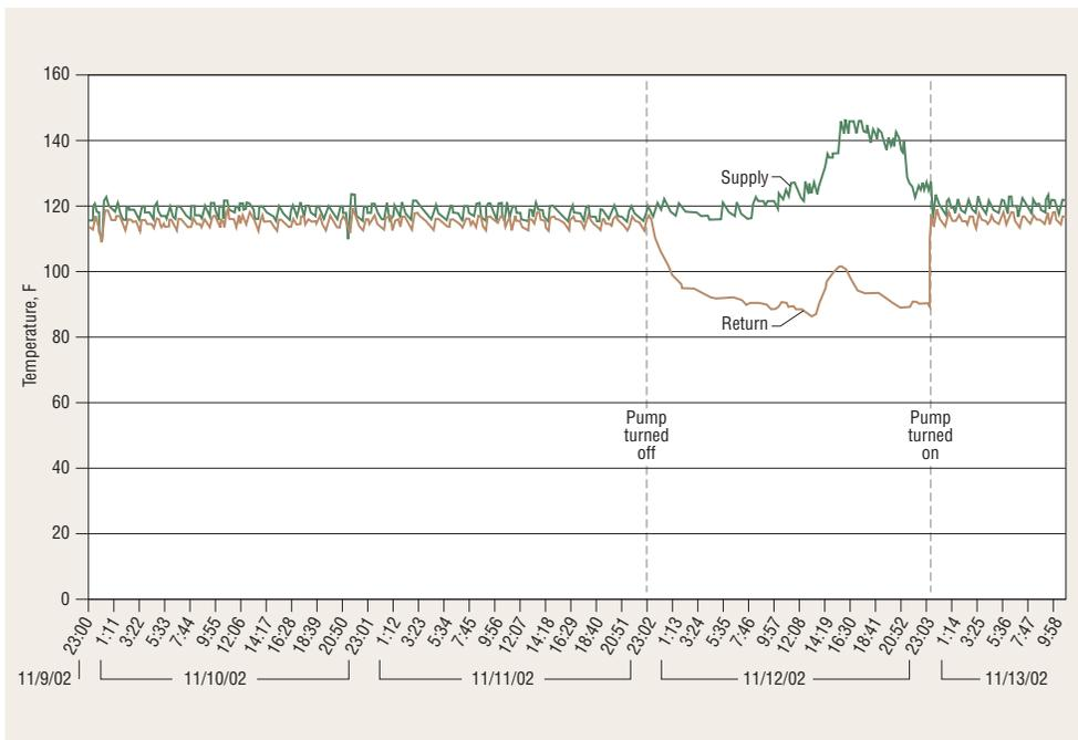
**FIGURE 1.** This building has an indirect water heater with an insulated 1/2-in. copper “fake” return piped back from the other end of the basement and a very small pump running nonstop. Just for a test, the return line pump was shut off at 11 pm and turned back on, after many complaints from tenants, nearly 24 hours later. The contrast between delivered temperature accuracy with and without the return line pump running is dramatic.
